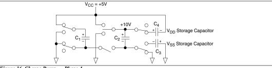
Figure 16. Charge Pump — Phase 4
