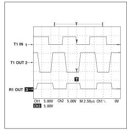
Figure 10. Driver Loopback Test Results at 235kbps
