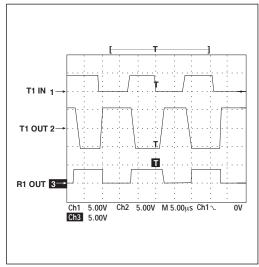
Figure 9. Driver Loopback Test Results at 120kbps
