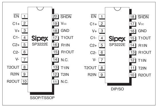
Figure 4. Pinout Configurations for the SP3222E
