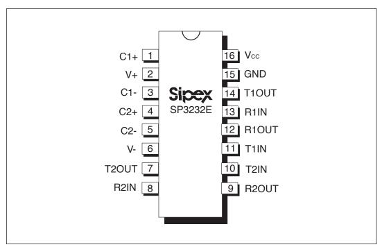
Figure 5. Pinout Configuration for the SP3232E
