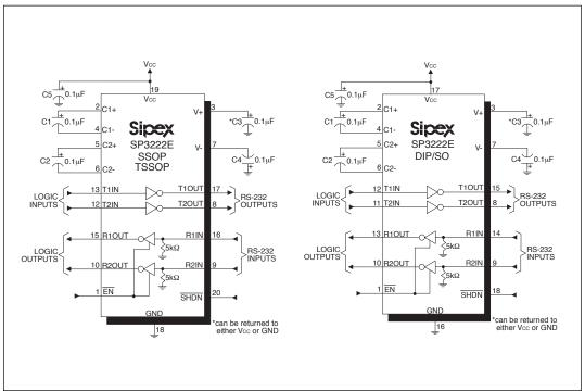
Figure 6. SP3222E Typical Operating Circuits
