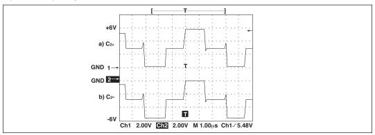
Figure 14. Charge Pump Waveforms
