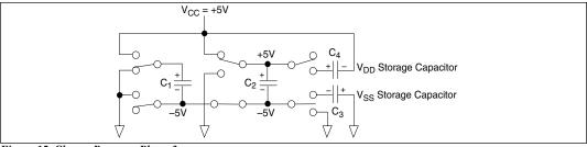
Figure 15. Charge Pump — Phase 3
