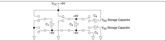
Figure 12. Charge Pump — Phase 1
