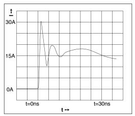
Figure 19. ESD Test Waveform for IEC1000-4-2
