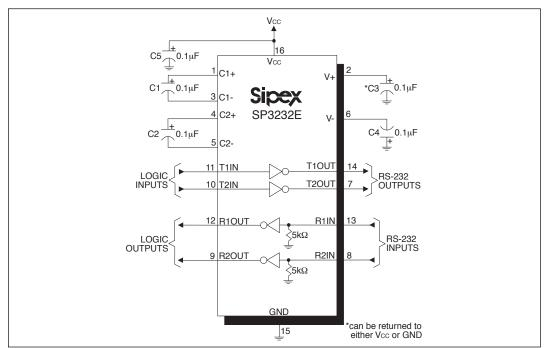
Figure 7. SP3232E Typical Operating Circuit
