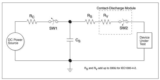
Figure 18. ESD Test Circuit for IEC1000-4-2
