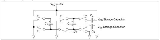
Figure 13. Charge Pump — Phase 2
