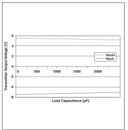
Figure 1. Transmitter Output Voltage VS. Load Capacitance for the SP3222 and the SP3232
