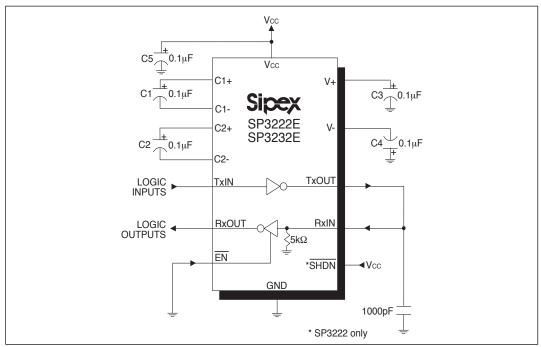
Figure 8. SP3222E/3232E Driver Loopback Test Circuit
