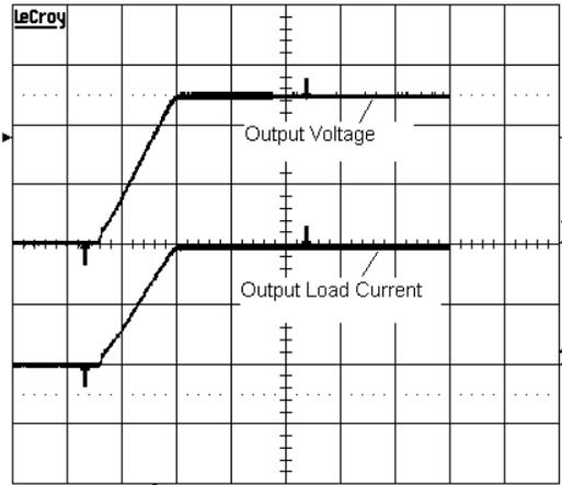
Load Transient Test ( $V_{IN}=5V$ ,  $V_{OUT}=1.2V$ ,  $I_{OUT}= 0A$  to  $4A$ , Forced Continuous Conduction Mode,  $L_{OUT}=1.3\mu H$ ,  $C_{OUT}=3x22\mu F$ , Channel 1: 50mV/Div, Channel 2: 5V/Div, Channel 4: 2A/Div, Time: 10µs/Div)
