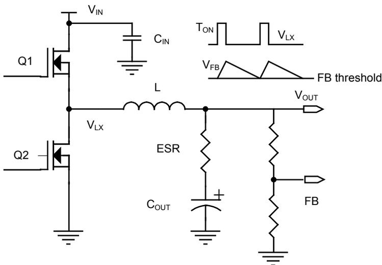
Figure 1 — PWM Control Method,  $V_{OUT}$  Ripple
