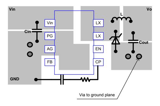
Figure 3. AOZ1014A (SO-8) PCB layout
