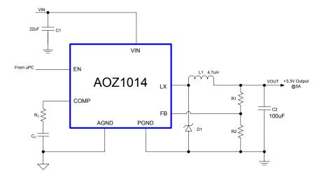
Figure 1. 3.3V/5A Buck Down Regulator
