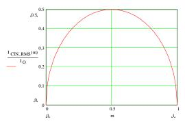
Figure 2. ICIN vs. voltage conversion ratio
