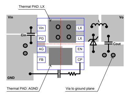
Figure 4. AOZ1014D (DFN-8) PCB layout
